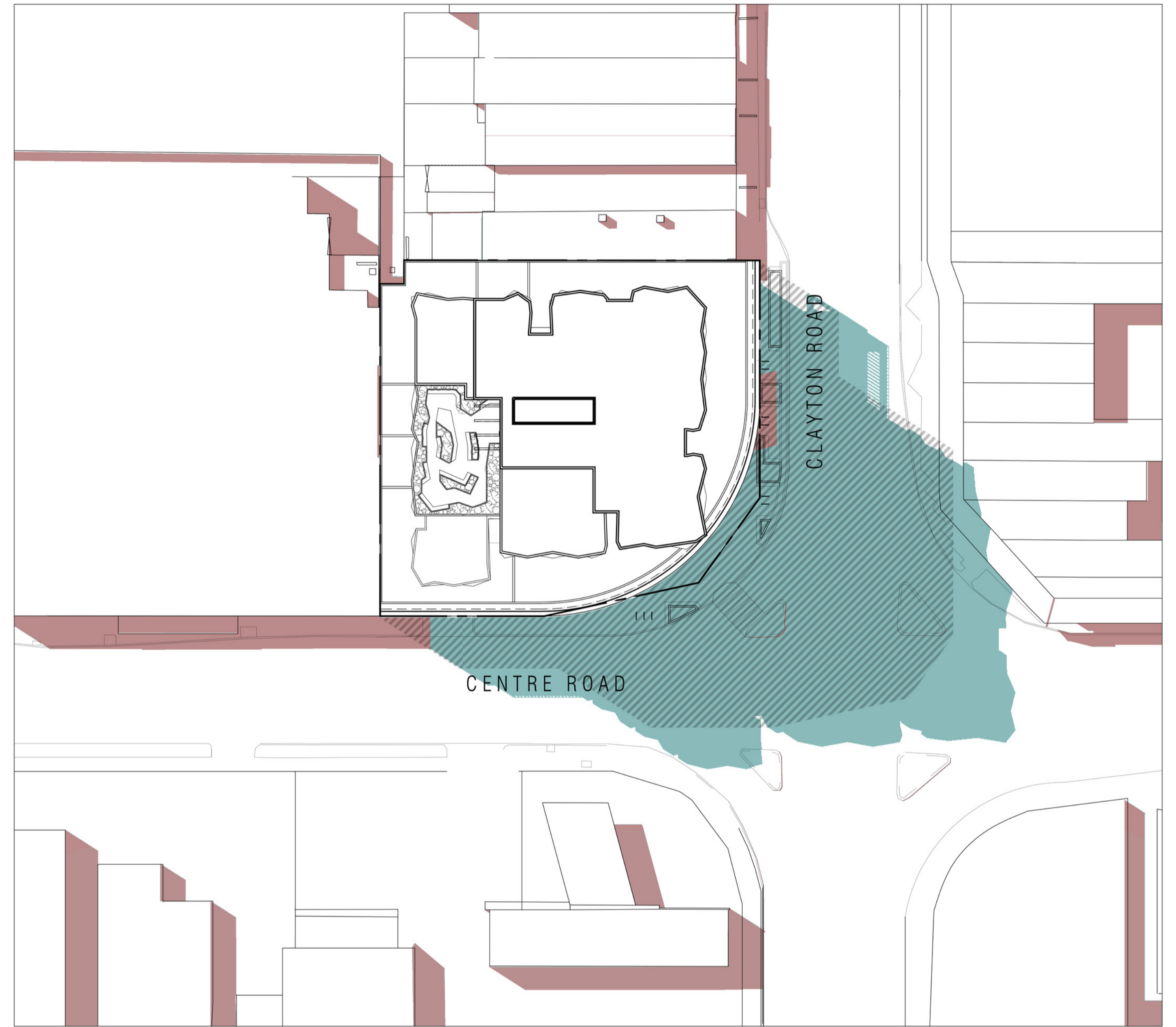
COMPARISON SHADOW DIAGRAM - 2PM, 22ND SEPTEMBER ■ EXISTING ■ PROPOSED ▨ 10 STOREY ENVELOPE IN LINE WITH CLAYTON PRECINCT PLAN
