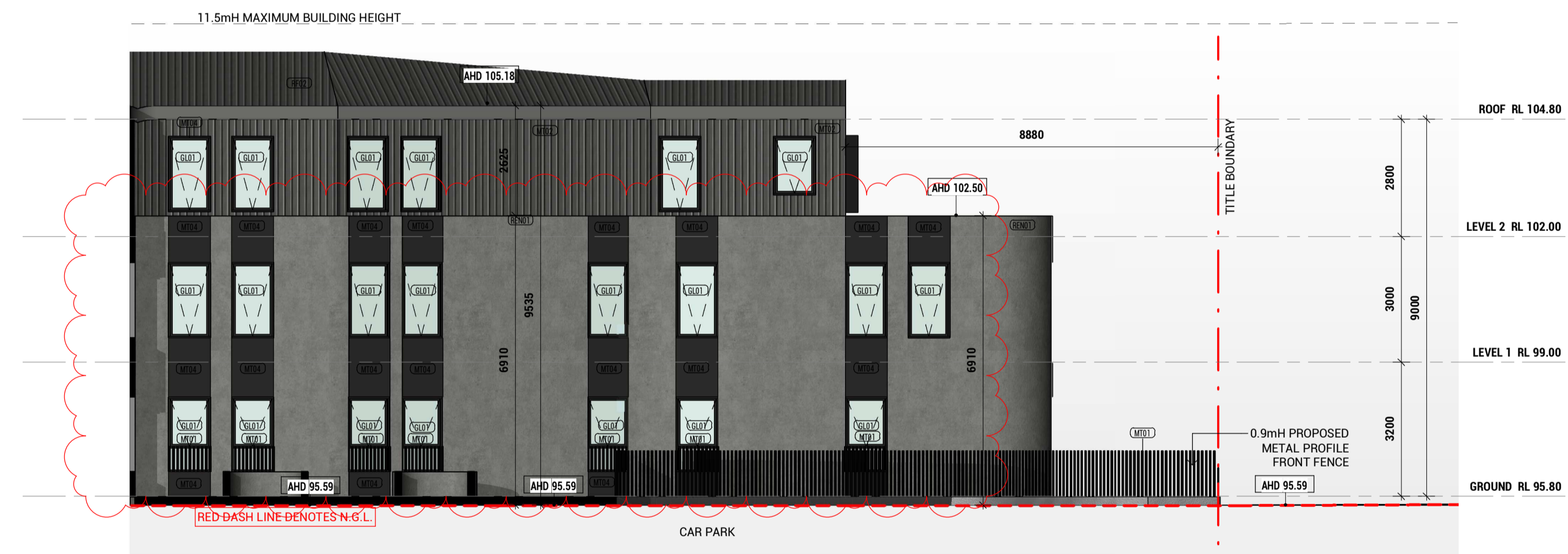
2 TP - South Internal Courtyard Elevation SCALE 1 : 100
