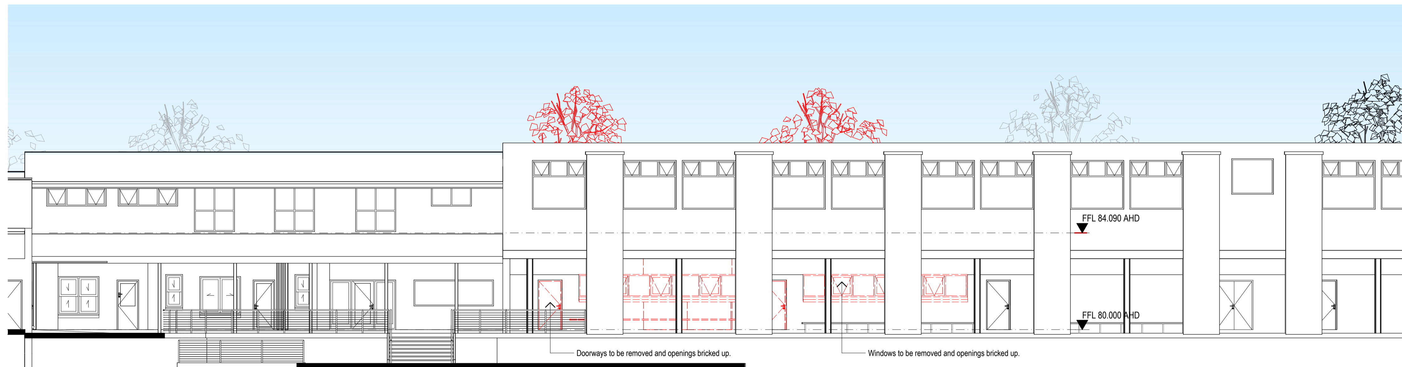
E4 South Elevation - Demolition 1:100
