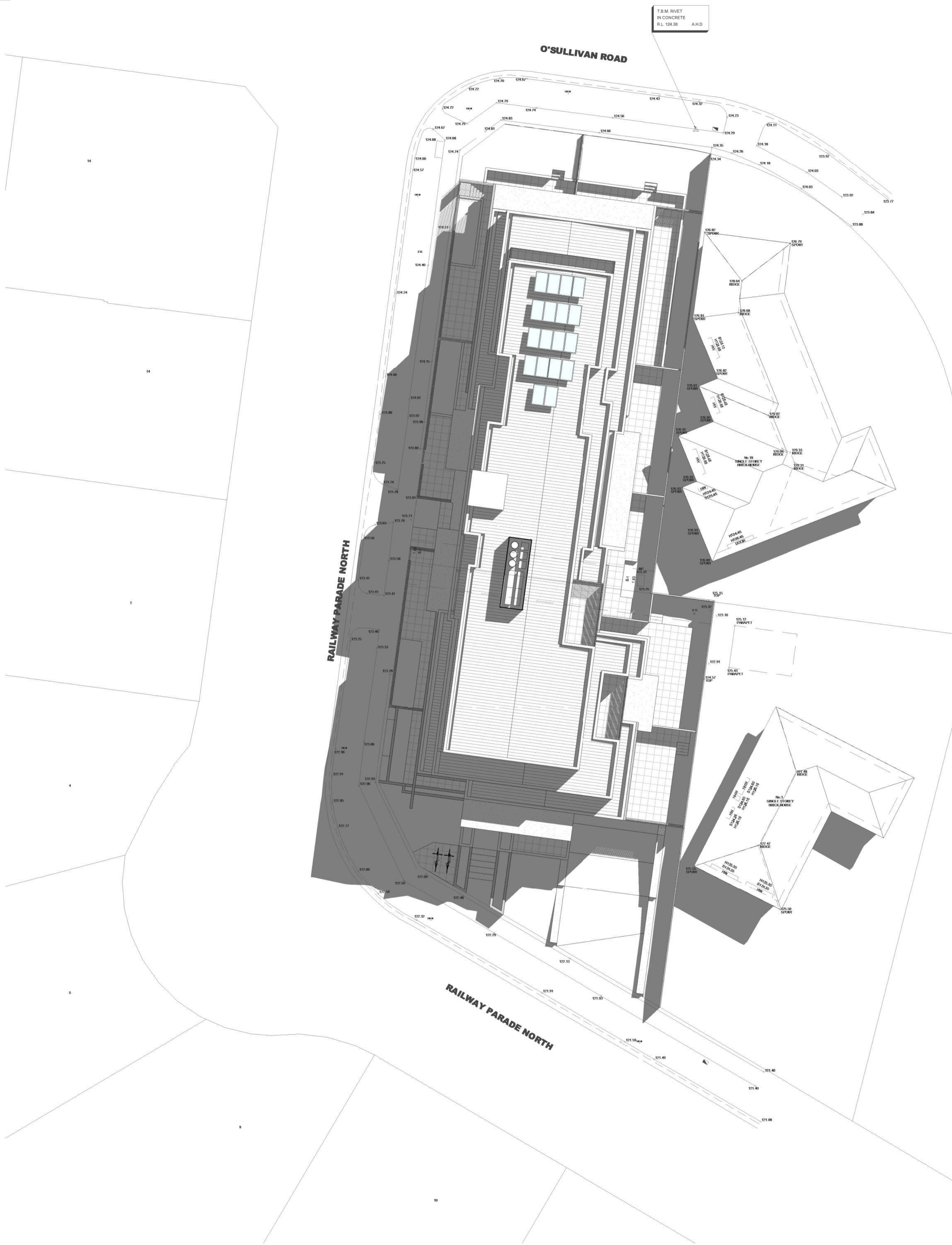
1 SHADOW DIAGRAM - SEP 22nd 10AM SCALE 1:200
