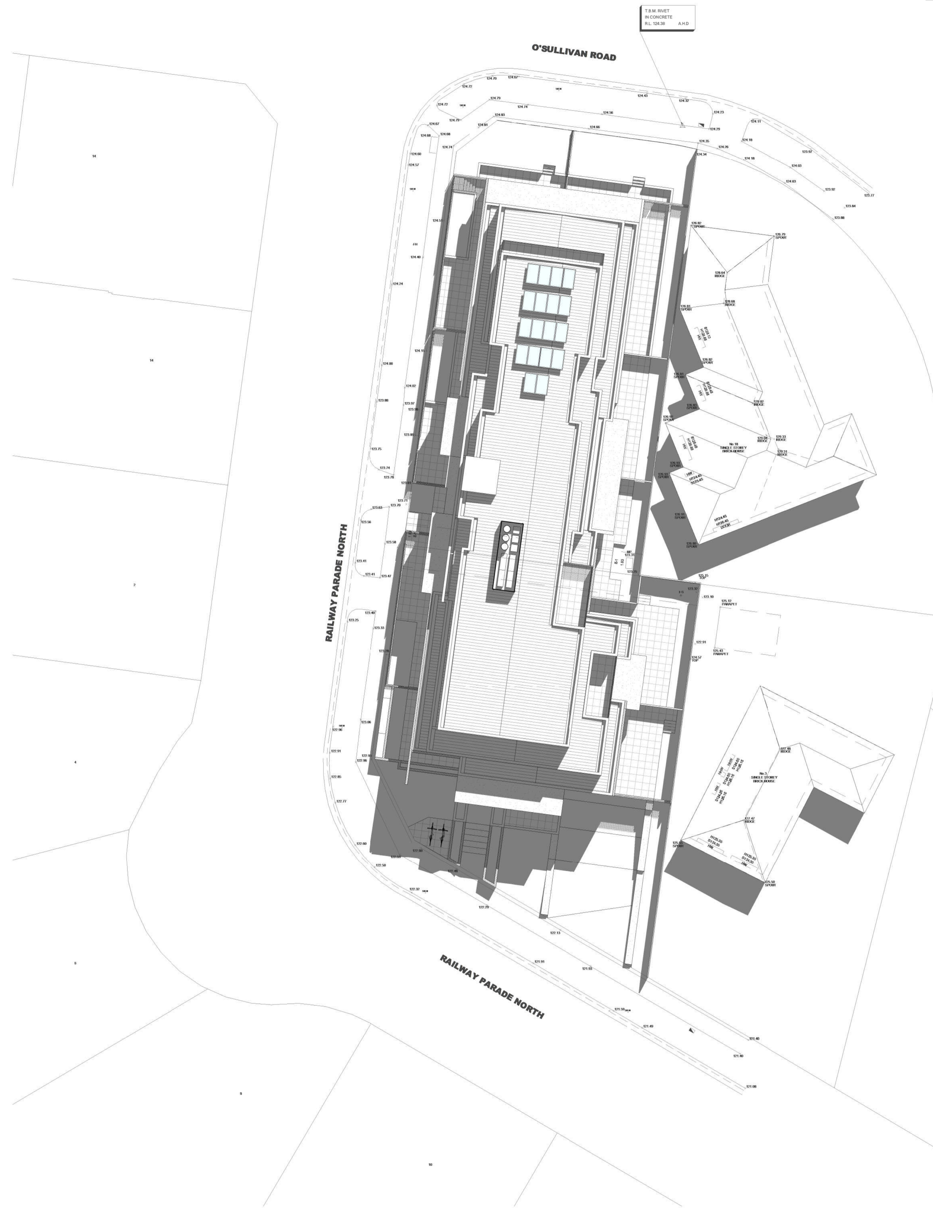
2 SHADOW DIAGRAM - SEP 22nd 11AM SCALE 1:200
