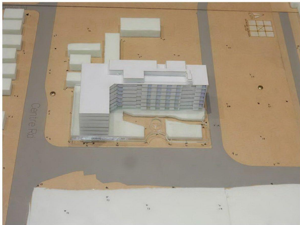
Figure 4 – Close-up view from the east of the 1/400 scale proposed The Links development in the wind tunnel.
