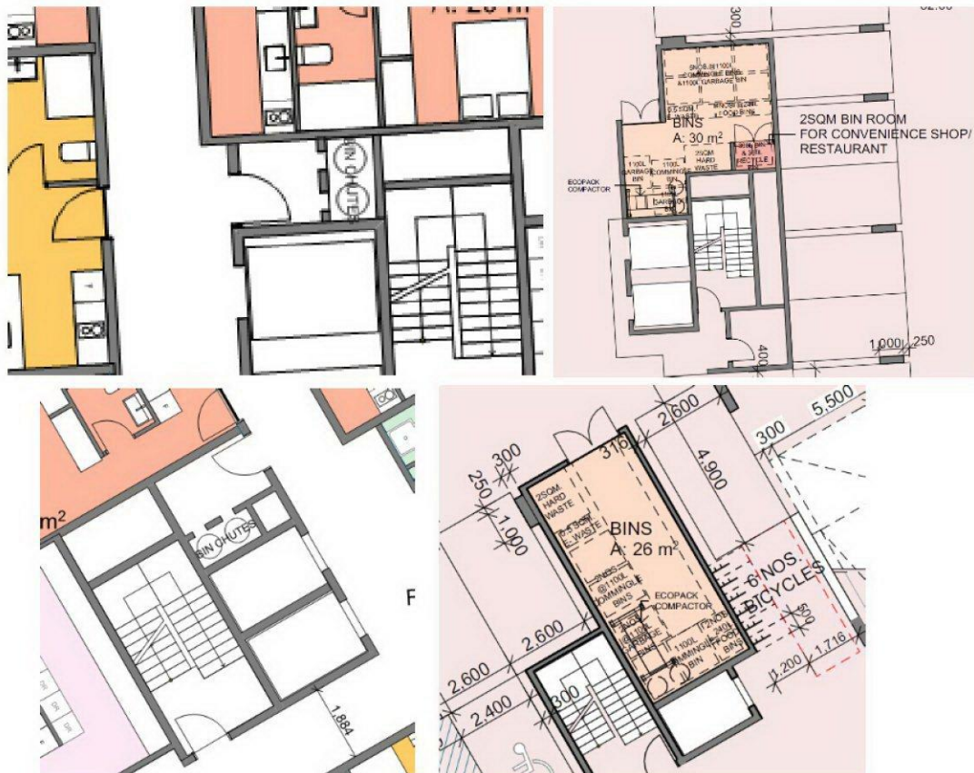
Figure 7 Waste chutes at each level and waste handling rooms in basement.
