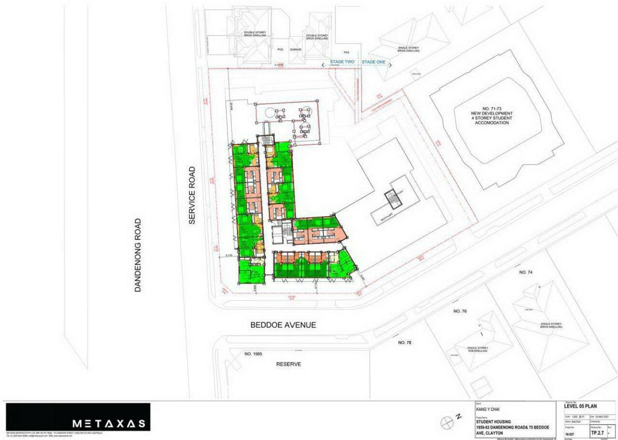
Figure 20 Daylight Plot, Fifth floor. Areas in green have a DF>2%.
