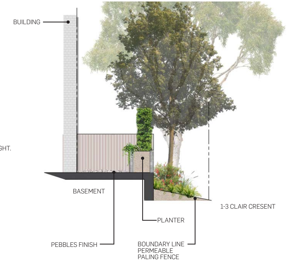
INDICATIVE SECTION (CC) OF BASEMENT 01 TERRACE
