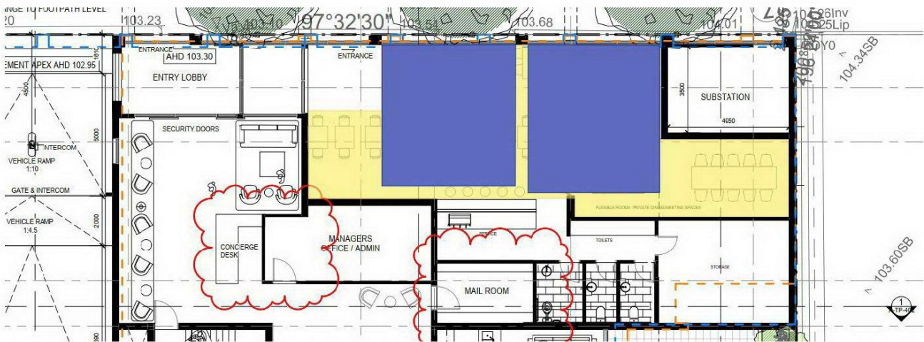
Figure 15: Daylight zone of compliance of the ground floor food and beverage premises of the development
