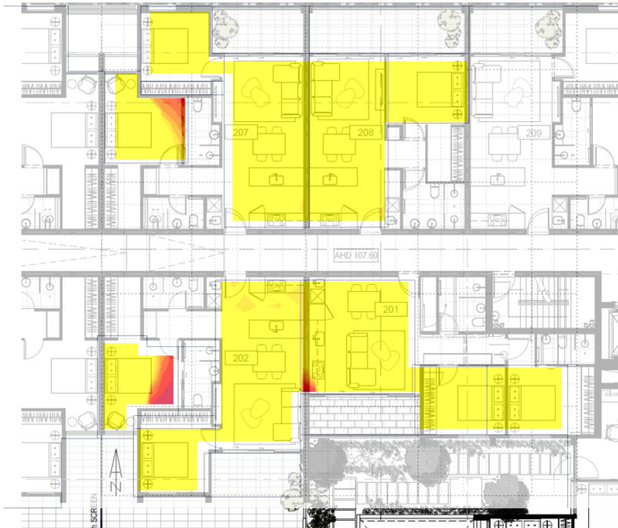
Figure 16: Daylight modelling results for the Level 1 main types of retirement village units
