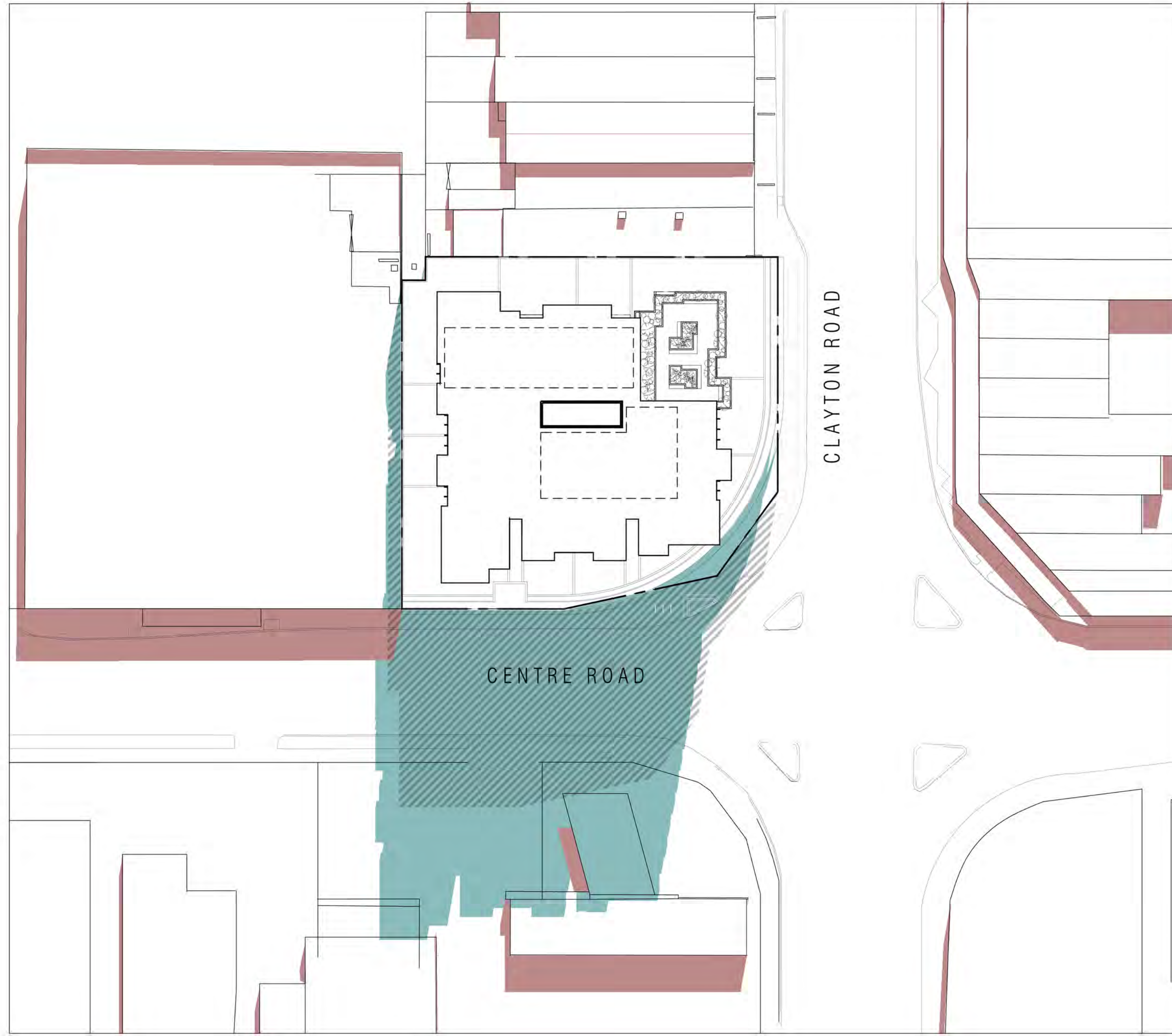
COMPARISON SHADOW DIAGRAM - 11AM, 22ND SEPTEMBER ■ EXISTING ■ PROPOSED ■ 10 STOREY ENVELOPE IN LINE WITH CLAYTON PRECINCT PLAN
