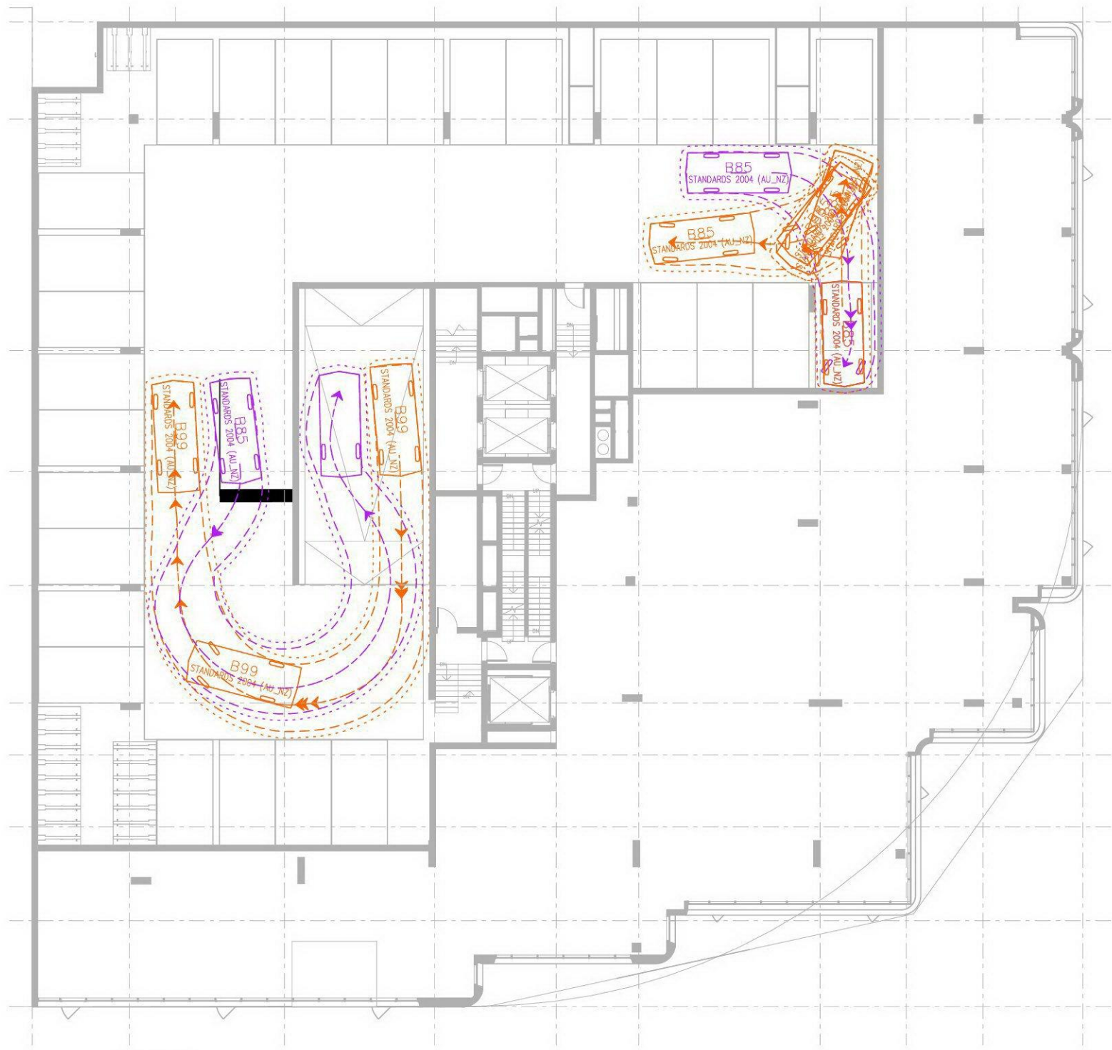
LEVEL 2 - - - - DESIGN VEHICLE SWEEP PATHS SHOWN DASHED ······ 300mm CLEARANCE ENVELOPE SHOWN DOTTED
