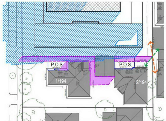
Extract of 10am shadow study showing acceptable impact of properties to the south
