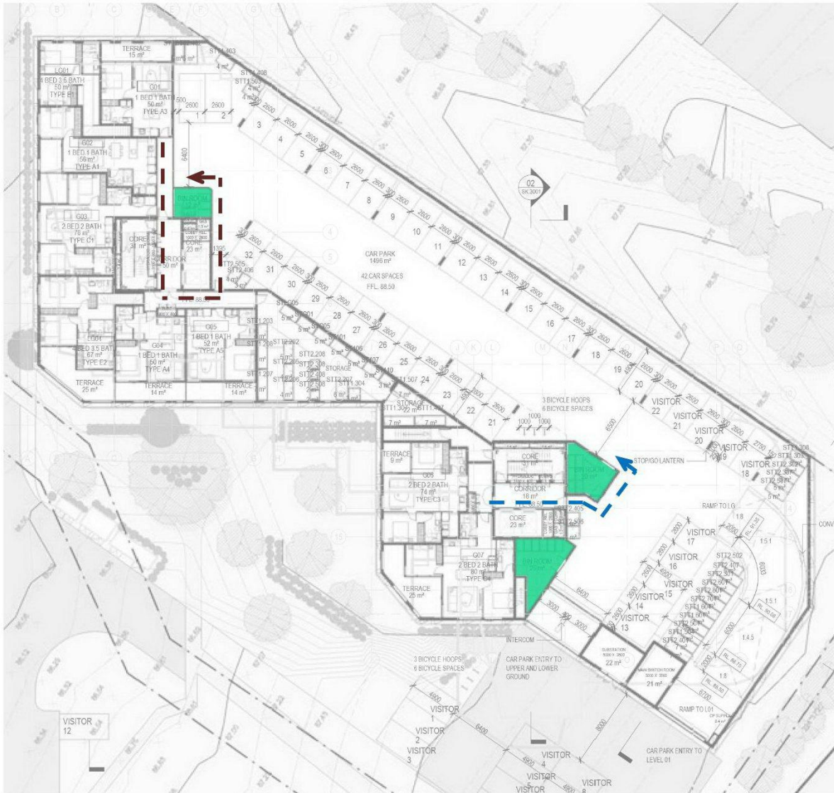
Figure 6: Residents' access to the allocated Bin Stores on Upper Ground Level (source: Cera Stribley)
