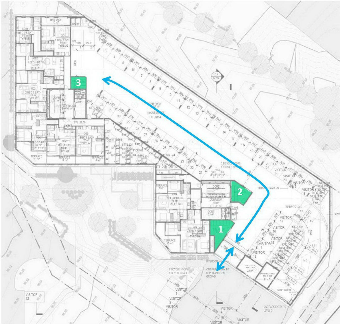
Figure 4: The Upper Ground Floor contains three Bin Stores. (1) Main Bin Store (2) Tower 2 Bin Store (3) Tower 1 Bin Store. Vehicular access into the area is on the south-eastern portion of the development. (source: Cera Stribley)
