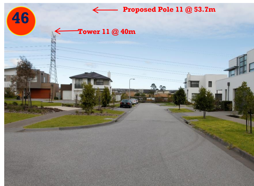
Figure 7 Photographic Analysis of the visual impact of the powerlines – Indicative location and size of the Proposed Overhead powerlines (VCAT 2014 plans) ( the coloured numbered circles correspond to the numbers in Figure 6)
