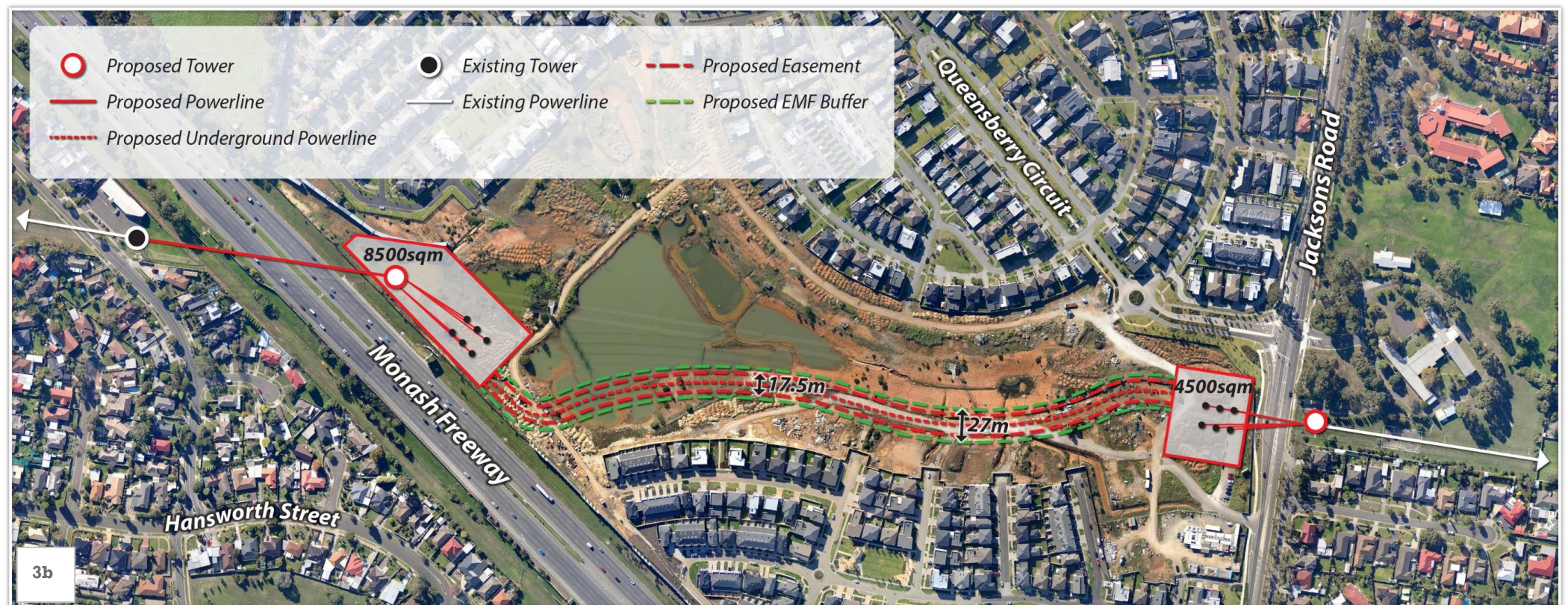
Figures 3b Diagram of the underground powerlines (endorsed plans 2.7.2013)
