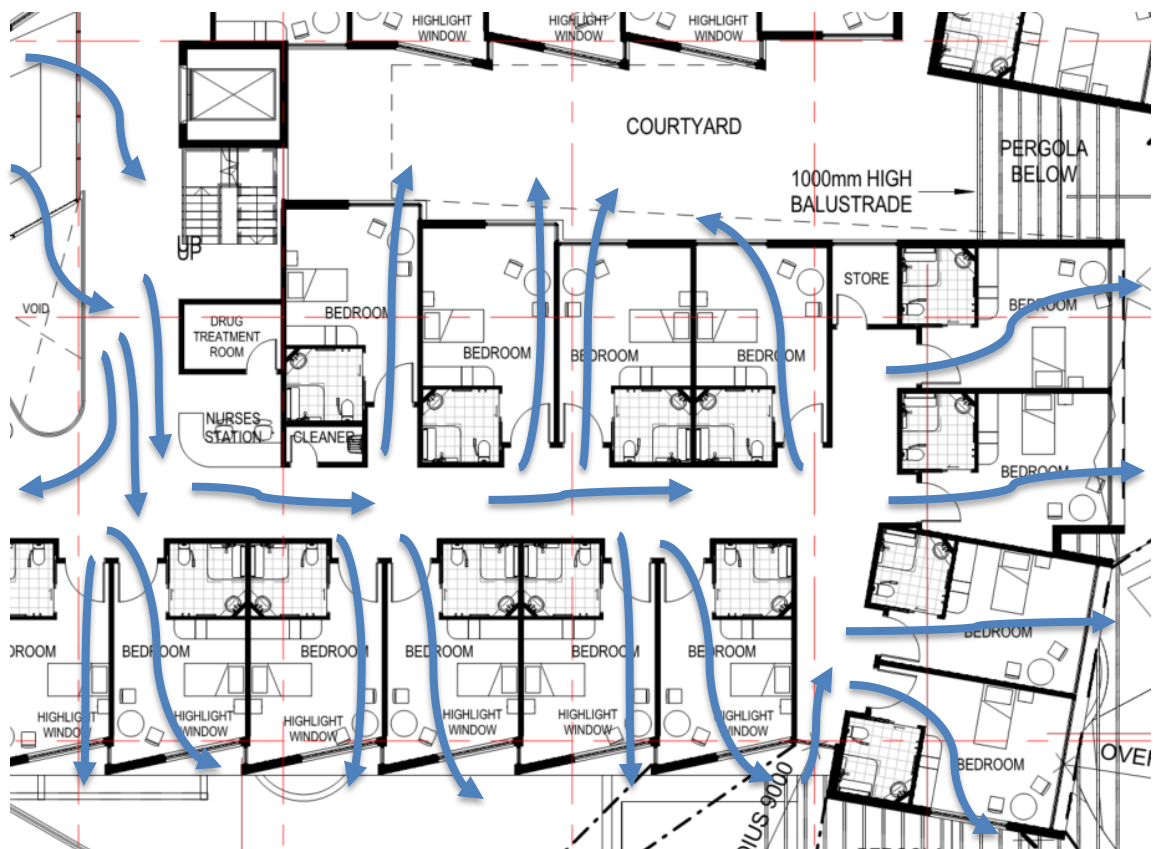
Figure 3.1 – Natural cross ventilation to aged care suites
