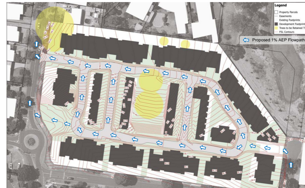
Figure 90. Proposed Finished Surface Levels - Ultimate Conditions
