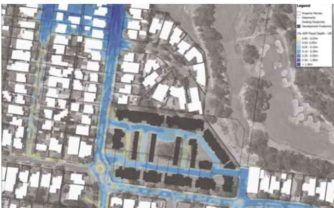
Figure 93. 1% AEP Flood Depth - Ultimate Conditions
