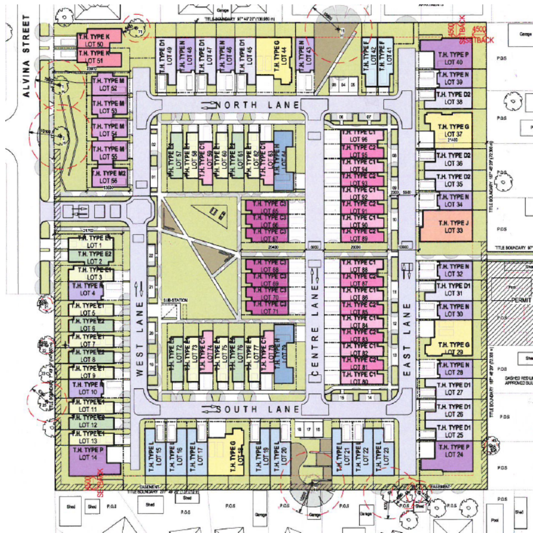
Figure 11 – Proposed development plan masterplan, drawing TP1.10 (source: Rothe Lowman)
