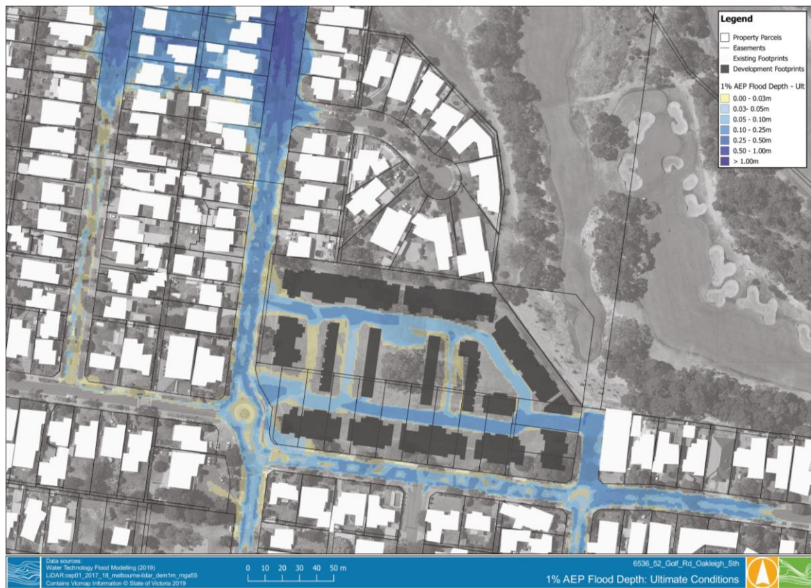
Figure 1-4 1% AEP Flood Depth – Ultimate Conditions
