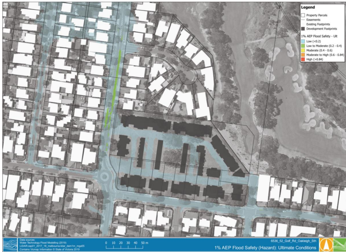
Figure 1-7 1% AEP Flood Safety (v.d ratio) – Ultimate Conditions
