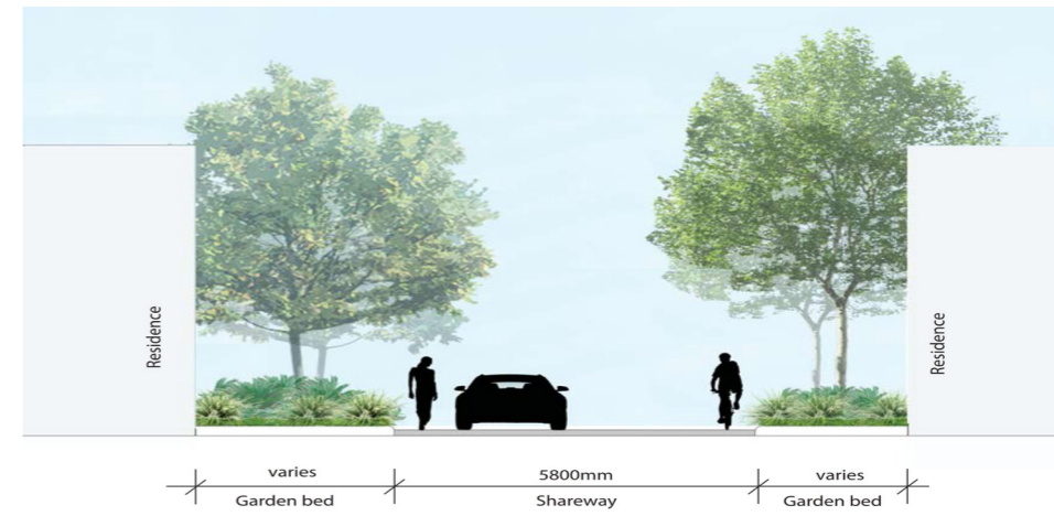
Figure 85. Internal shareway road section
