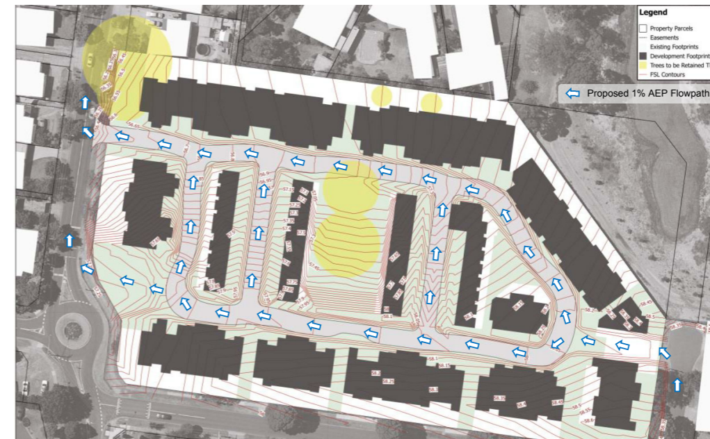
Figure 90. Proposed Finished Surface Levels - Ultimate Conditions
