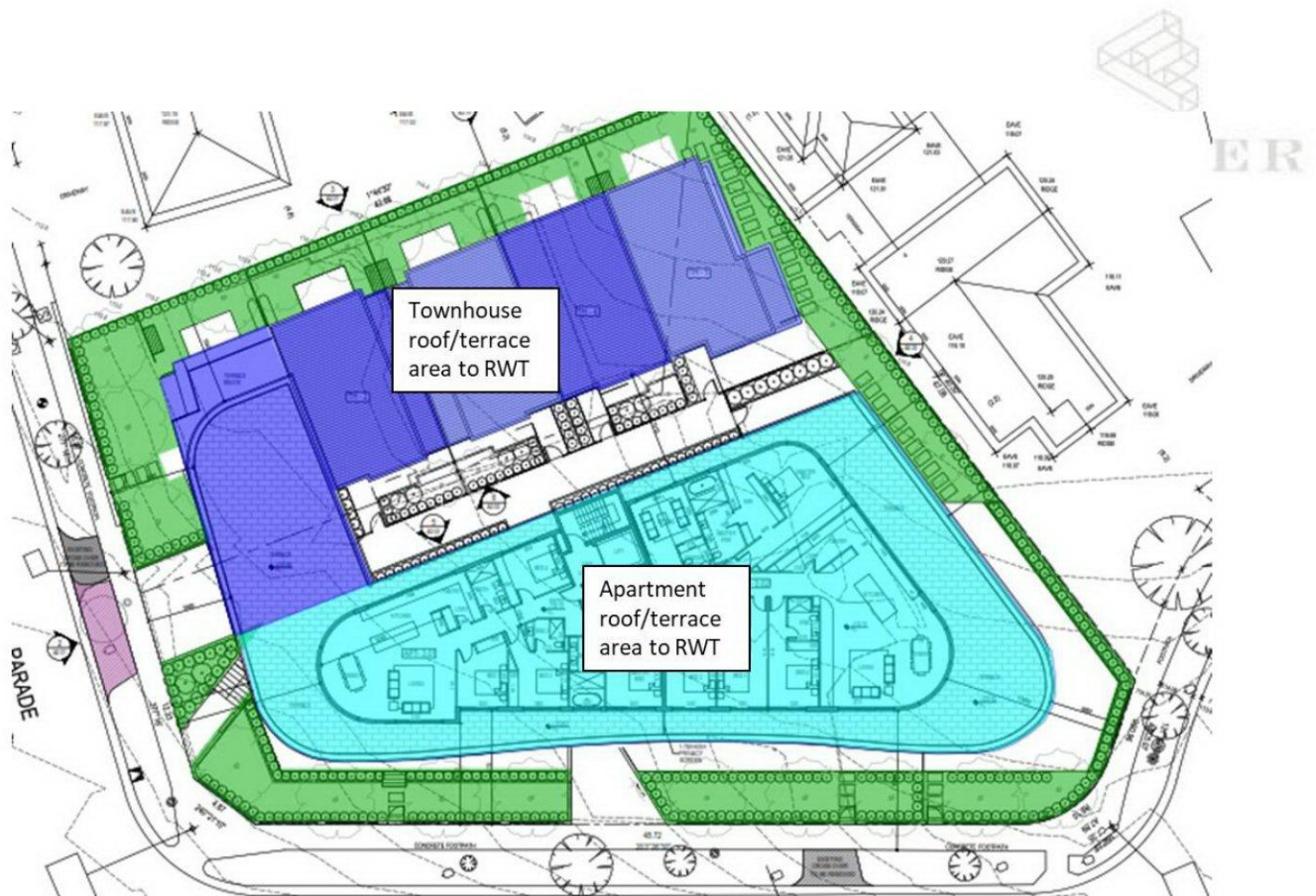
Figure 4: Roof catchment area to rainwater tank (blue), permeable area (green) and untreated impervious areas (white/clear) for the development.
