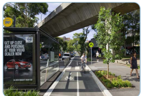
Bidirectional separated cycleway: Bourke Street, Sydney NSW
