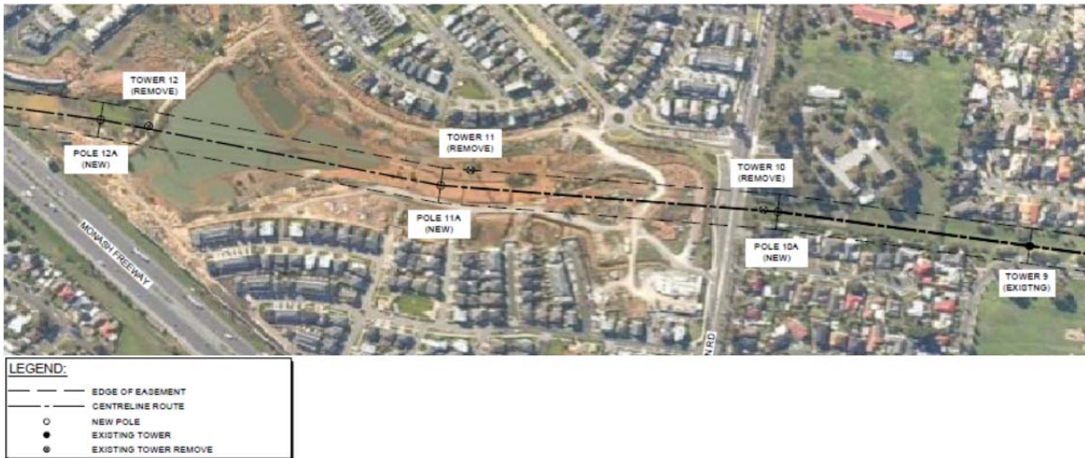
Figure 3 Proposed Deviation using Steel Poles (excerpt from drawing 60327503-SHT-00-EL-1001-A)
