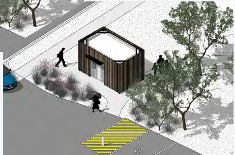
Below: stainless steel automated unit with timber cladding.
