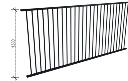
FENCE TYPE 1: FN2 DESCRIPTION: OPEN METAL FENCE COLOUR: BLACK POWDERCOAT FINISH LOCATION: FRONT, SIDE & REAR BOUNDARIES
