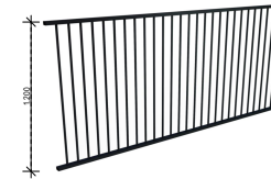
FENCE TYPE 1: FN1 DESCRIPTION: OPEN METAL FENCE COLOUR: BLACK POWDERCOAT FINISH LOCATION: FRONT BOUNDARY.
