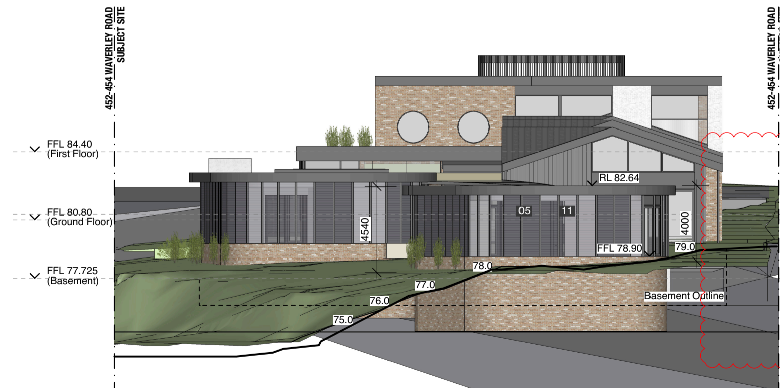
4 South-West Elevation (Boundary Line) Scale: 1:200
