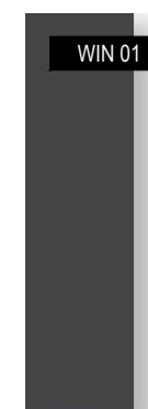
ALUMINIUM WINDOW FRAMES Powder Coated Finish: To Match Colorbond 'Monument' (or similar)
